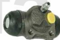
5. 673 199 links/rechts left/right Ø 17,46 mm System: Sumitomo
