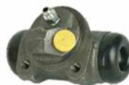
6. 673 559 rechts/right System: Bendix Ø 19,05 mm + 4x4
